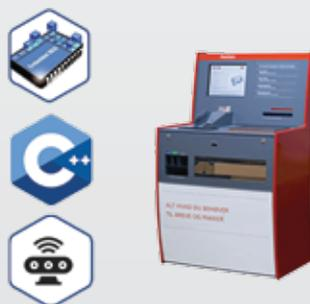
**Embedded software for SPU (Self Post Unit)** using C++ and desktop application. The SPU measures and weighs letters and parcels for domestic or foreign destinations, and calculates the postage.
