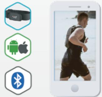
**iOS & Android fitness App.** It pulls data from a heart rate monitor called Polar H7 via Bluetooth, synchronizes with the central system, and presents statistics to the end user for improvements on daily workout routines.
